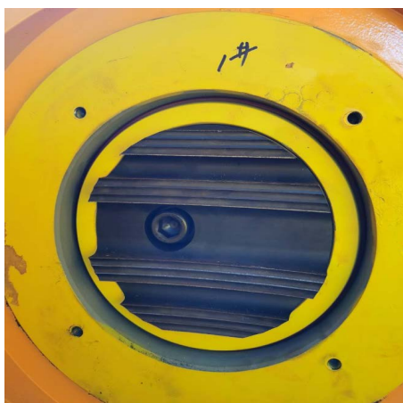
Figure 4. The clam fixed on the front end of the piston of the hydraulic cylinder 图 4. 卡爪固定于液压缸活塞前端
