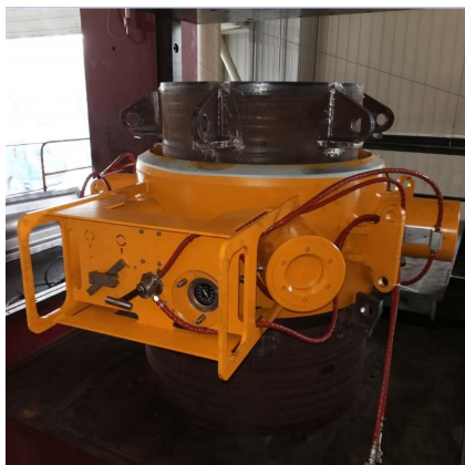
Figure 7. 42-inch pile gripper and load test
