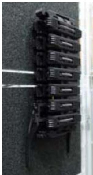
Figure 18. Wall-climbing robot with spiny grippers [25]
