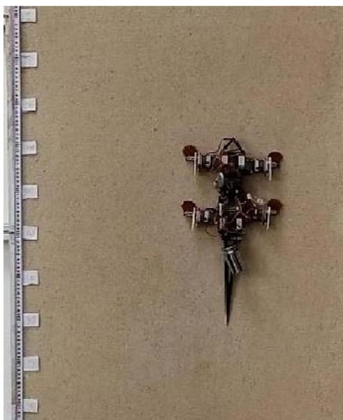
Figure 17. Quadruped wall-climbing robot [24]
