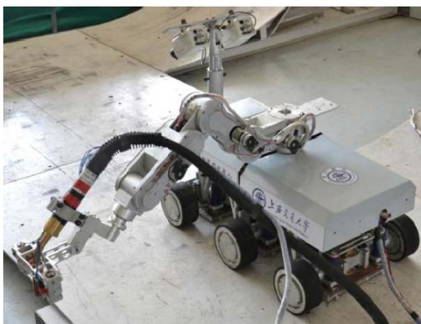
**Figure 10.** Magnetic adhesion welding robot [15]
