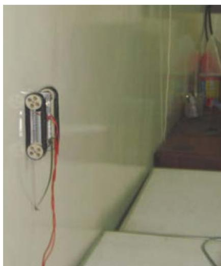
**Figure 27.** Tank-like Climbing Robot [39]
