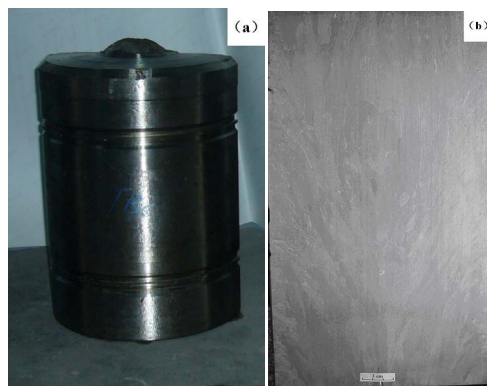
Figure 2. TC4 titanium alloy ingot morphology (a) and alloy plate photograph (b)
