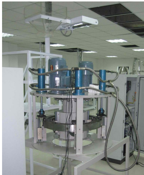
Figure 2. The photograph of BF distributor device for training teaching
