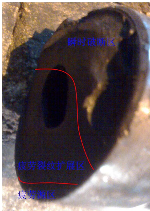
Figure 3. Fracture picture of the percussion shaft 图 3. 打击轴断口照片
