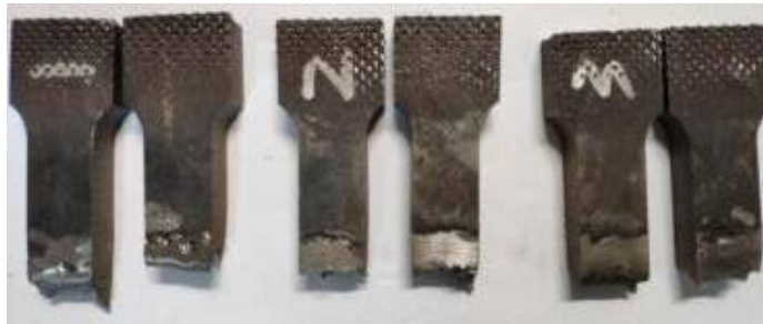
Figure 4. Specimen after tension 图 4. 拉伸后试样
