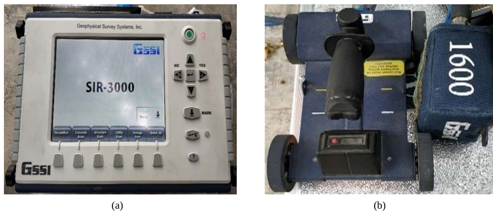
Figure 4. (a) SIR-3000 ground penetrating radar main engine; (b) 1600 M antenna 图 4. (a) SIR-3000 探地雷达主机; (b) 1600 M 天线
