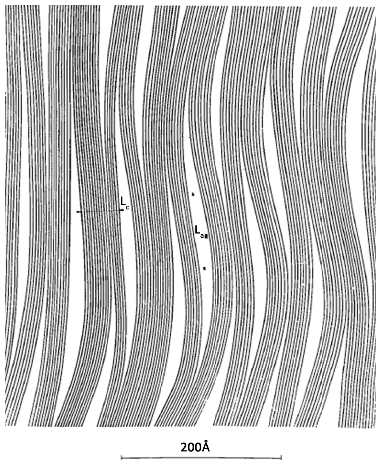
Figure 7. Schematic representation of the structure of carbon fibres [9]
