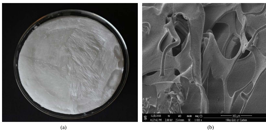
Figure 1. (a) Photographs of SA/CMC, (b) SEM images of SA/CMC 图 1. (a) SA/CMC 光学照片; (b) SA/CMC 扫描电镜照片
