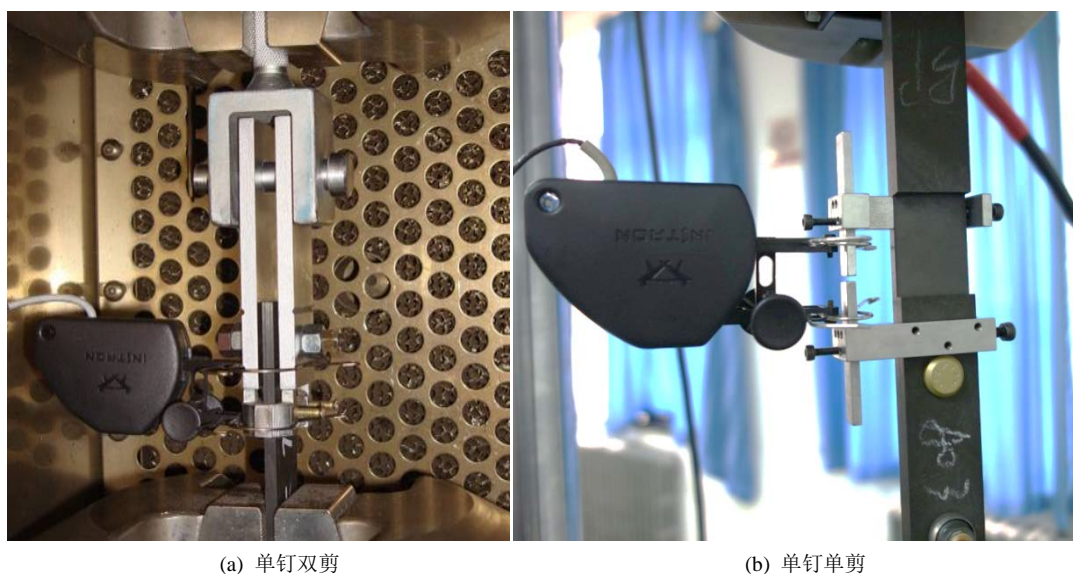
Figure 1. Photo: strength test state of single nail double shear and single nail single shear connection 图 1. 单钉双剪和单钉单剪连接强度试验状态照片
