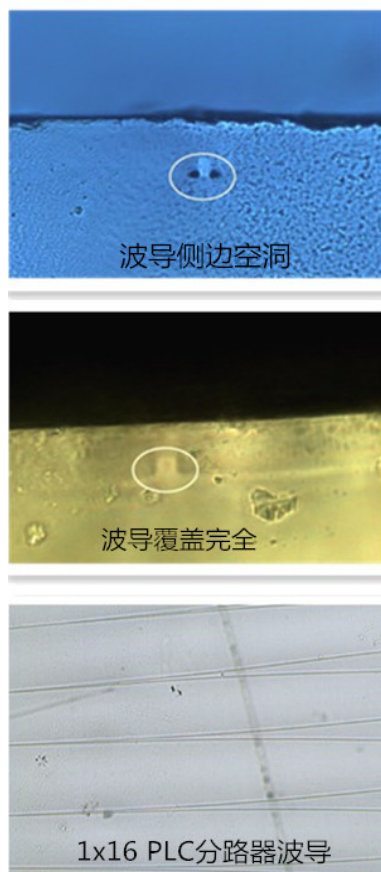
Figure 10. FHD cladding layer appearance: (a) hollow on side of waveguide (b) cladding properly covered (c) 1 \times 16 PLC splitter waveguide pattern 图 10. FHD 上包层形貌(a)波导侧空洞, (b)上包层覆盖完全, (c) 1 \times 16 PLC 分路器波导图案
