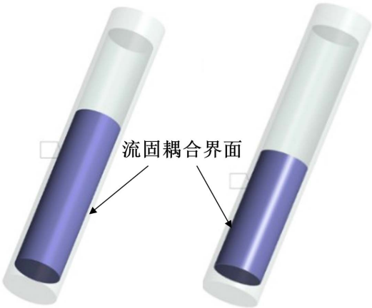
Figure 5. Definition of fluid-solid coupling interface in the accumulator barrel 图 5. 蓄能器筒体流固耦合界面定义
