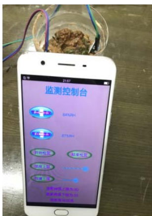
Figure 13. Humidity exceeds the preset value 图 13. 湿度超出预设值
