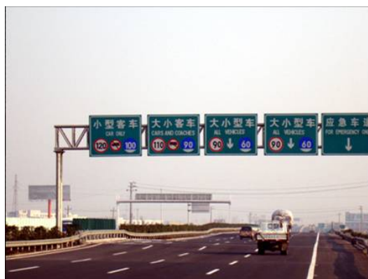
Figure 8. Speed limit by the lane and motorcycle type (reference case) 图 8. 分车道、分车型限速(参考案例)
