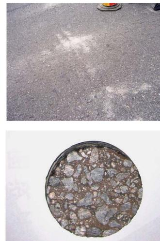
**Figure 6. The sections of purt thick liquid of road surface**
