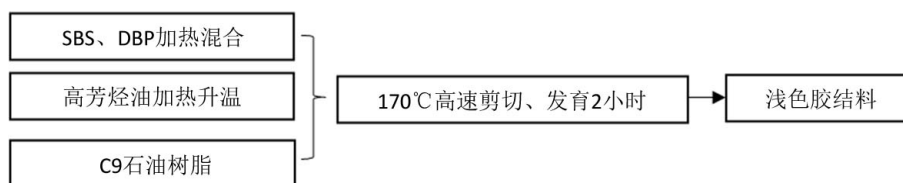
Figure 1. Technical route of preparation of light-colored asphalt binder 图 1. 浅色胶结料的制备技术路线
