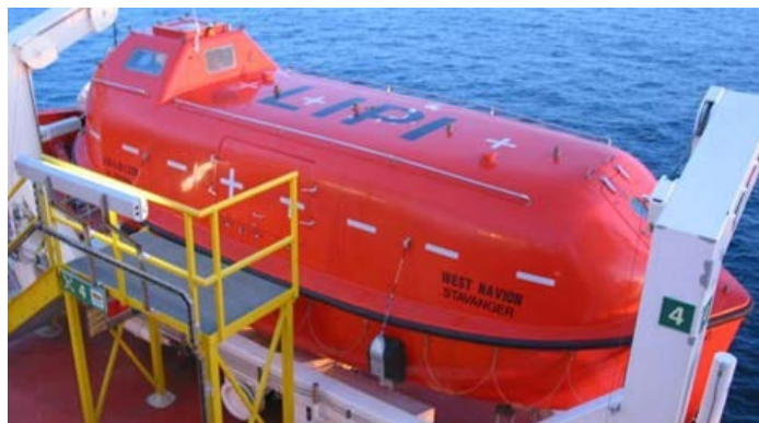
Figure 3. Existing escape equipment or device—lifeboat
