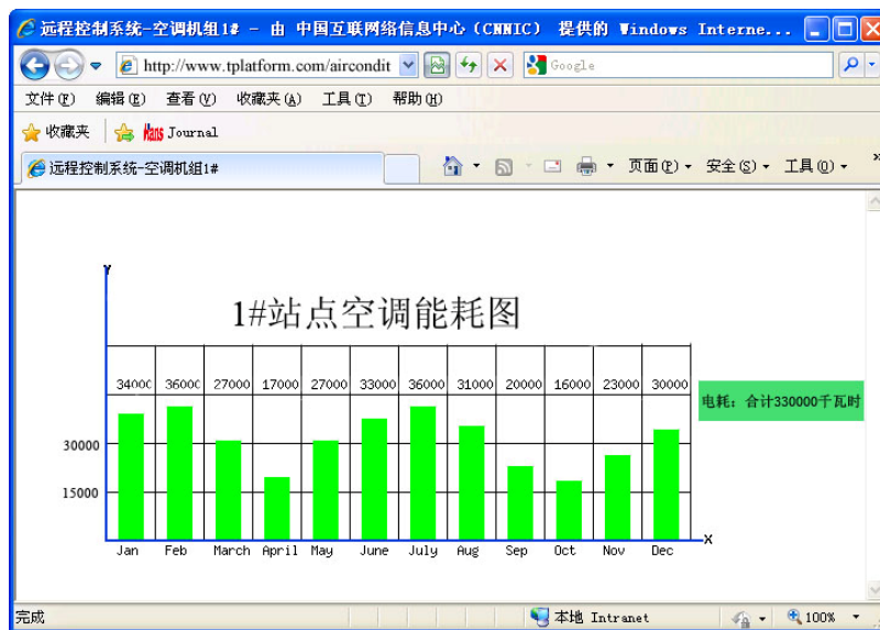
Figure 6. Central air conditioning unit energy consumption figure 图 6. 中央空调机组能耗图
