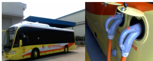
Figure 1. The interface for fast charging technique of the bus 图 1. 重庆快速充电客车及充电接口
