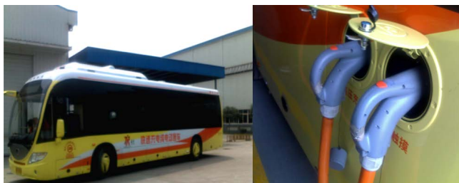
Figure 8. Chongqing Hengtong fast charging bus and the power-charging connector
