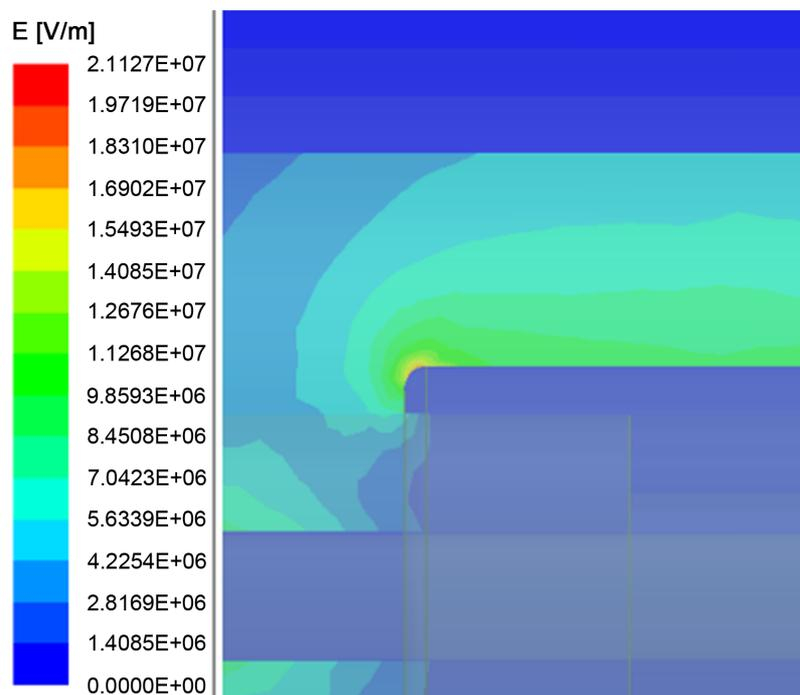
**Figure 23.** Electric field at the inner shield of 35kV power cable quick-plug connector
