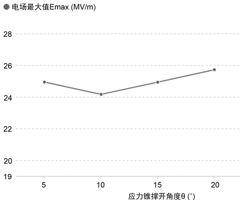
**Figure 6.** Influence of stress cone opening angle on the magnitude of electric field
