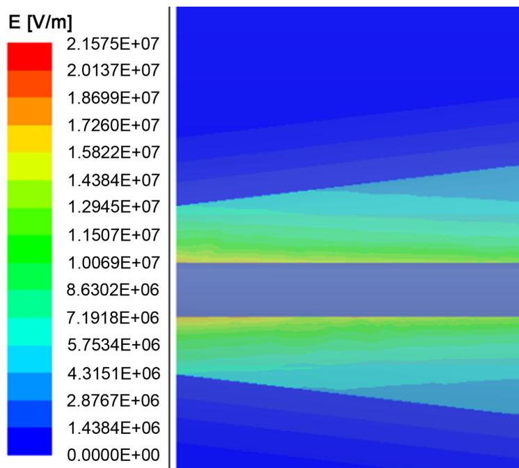
**Figure 9.** Electric field at the stress cone of the 35kV power cable push-in connector
