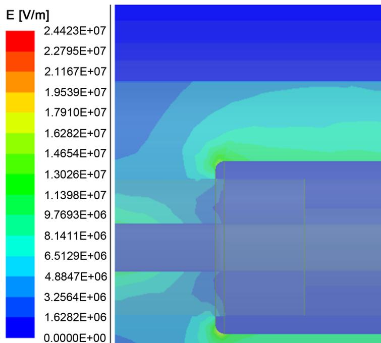
Figure 26. Electric field at the inner shield of 35kV power cable quick-plug connector
