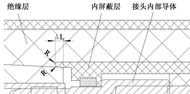
Figure 17. Structural diagram of the inner shield of the 35kV power cable quick-plug connector
