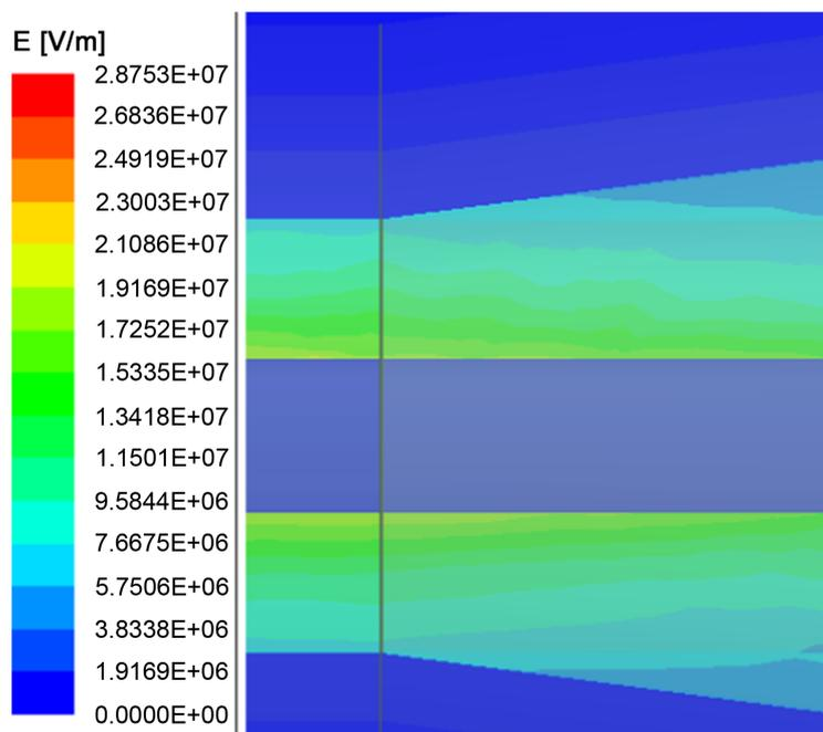
**Figure 15.** Electric field at the stress cone of the 35kV power cable push-in connector
