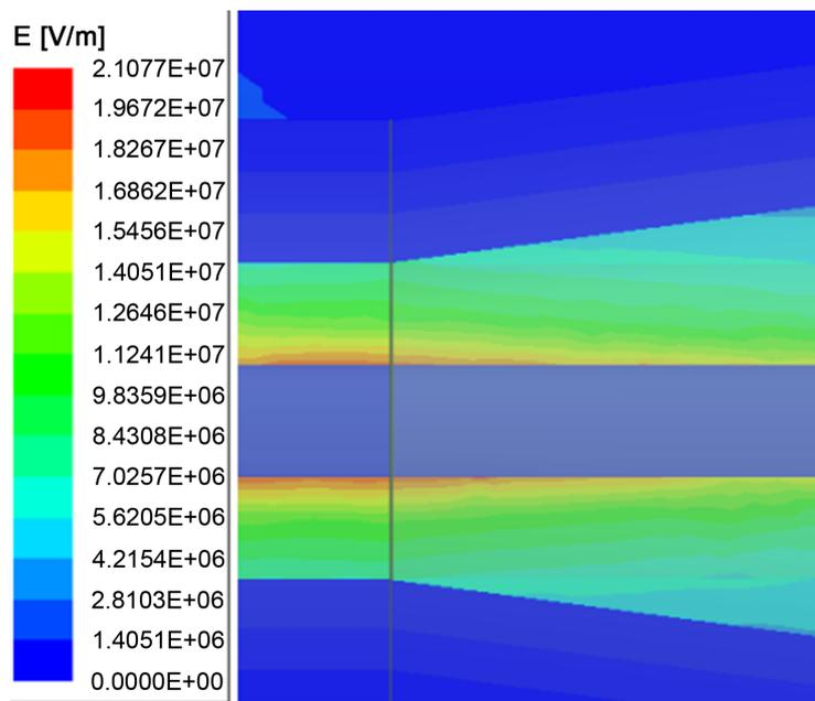
**Figure 13.** Electric field at the stress cone of the 35kV power cable push-in connector
