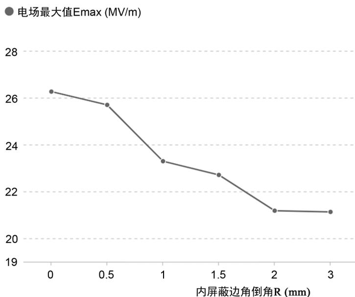
**Figure 24.** Influence of chamfering of inner shielding layer on the magnitude of electric field
