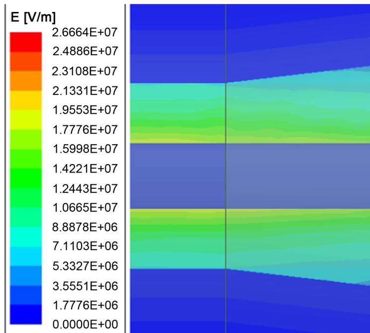
**Figure 14.** Electric field at the stress cone of the 35kV power cable push-in connector
