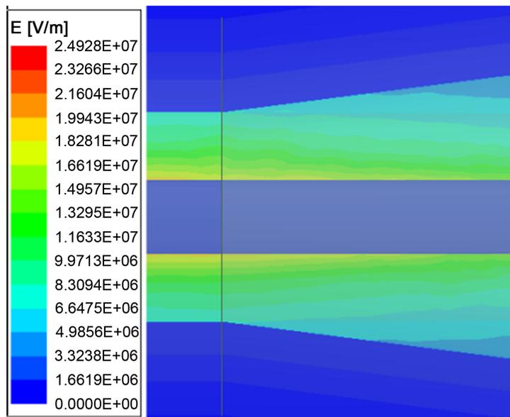
**Figure 4.** Electric field at the stress cone of the 35kV power cable push-in connector
