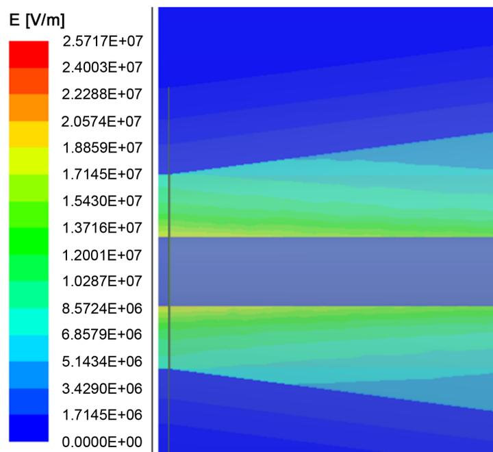
**Figure 5.** Electric field at stress cone of 35kV power cable push-in joint
