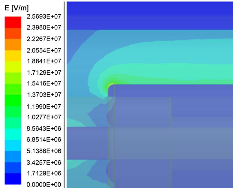
**Figure 19.** Electric field at the inner shield of 35kV power cable quick-plug connector
