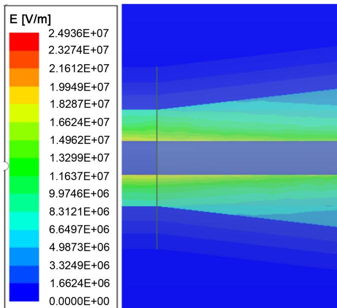
Figure 2. Electric field at the stress cone of 35kV power cable push-in joint
