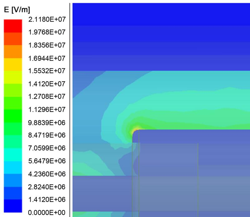
Figure 22. Electric field at the inner shield of 35kV power cable quick-plug connector
