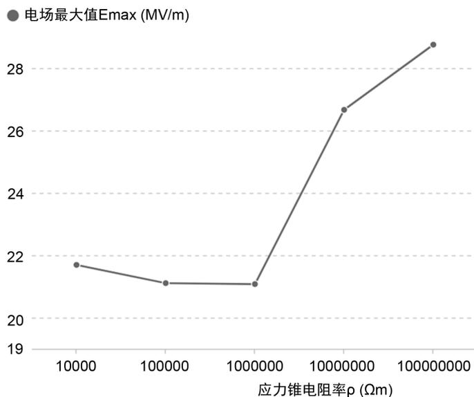
Figure 16. Effect of stress cone resistivity on electric field magnitude
