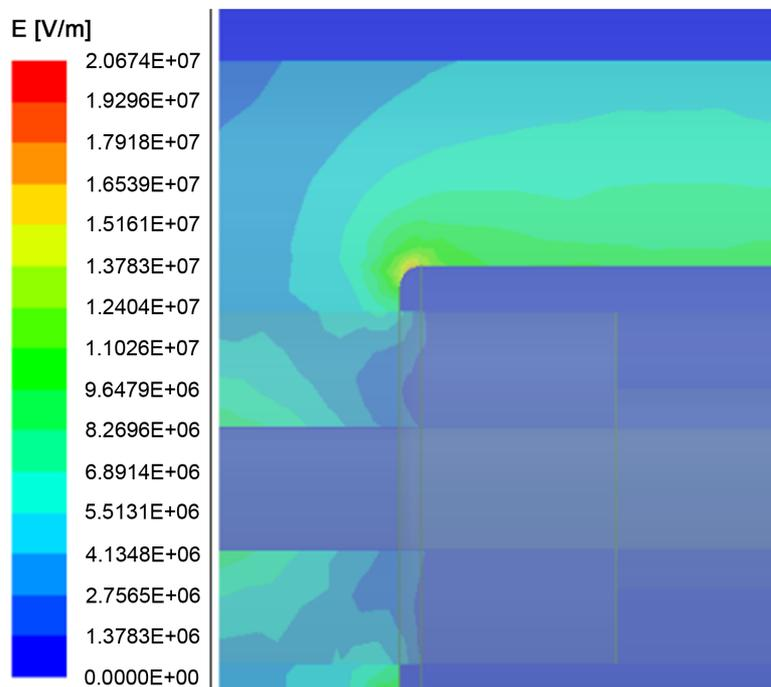
Figure 27. Electric field at the inner shield of 35kV power cable quick-plug connector
