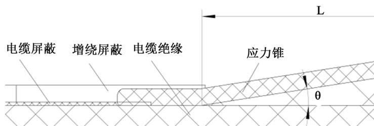
Figure 1. Structure diagram of stress cone of quick-plug joint of 35kV power cable
