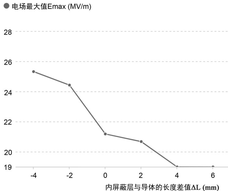
Figure 30. Influence of the difference between the inner shielding layer and the conductor length on the magnitude of the electric field
