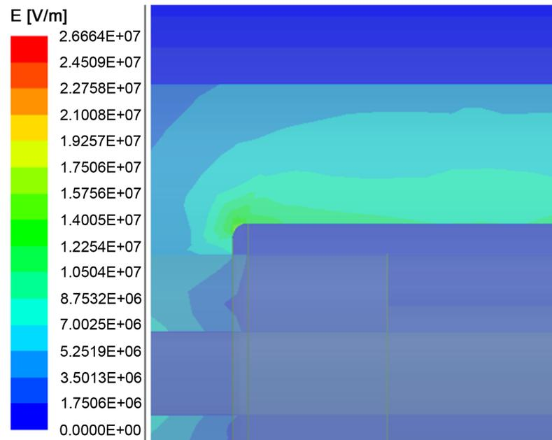
Figure 18. Electric field at the inner shield of 35kV power cable quick-plug connector
