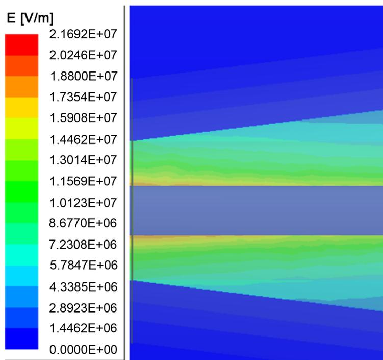
**Figure 8.** Electric field at the stress cone of the 35kV power cable push-in connector
