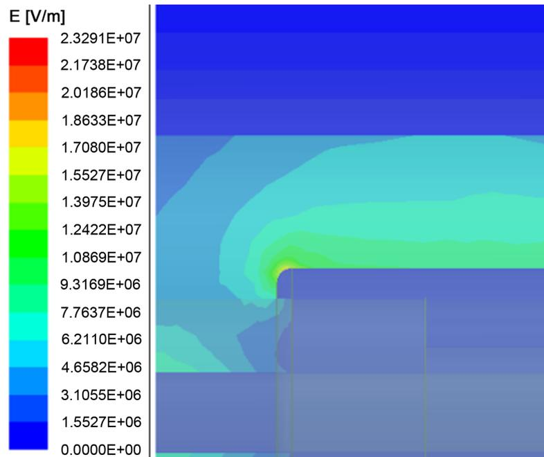
**Figure 20.** Electric field at the inner shield of 35kV power cable quick-plug connector
