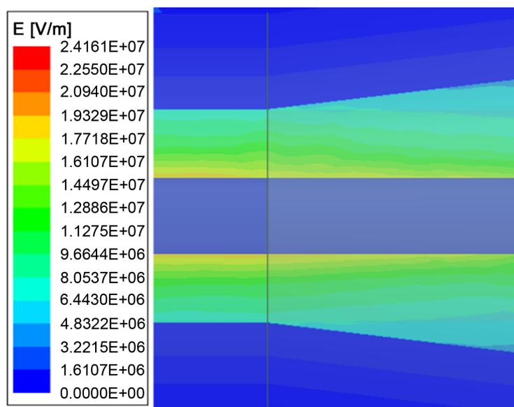
Figure 3. Electric field at the stress cone of the 35kV power cable push-in connector
