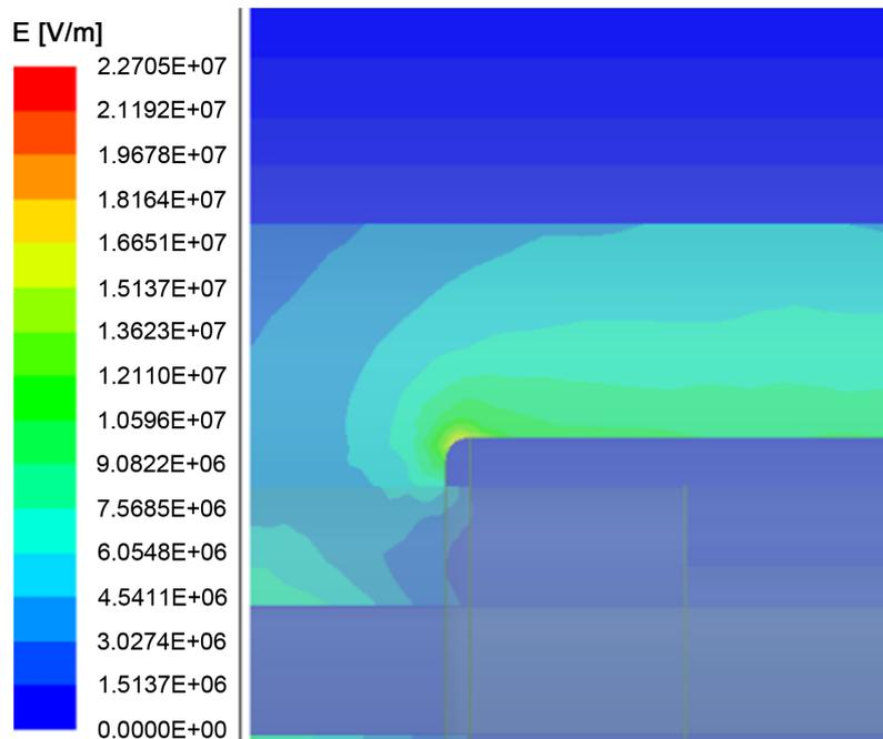
Figure 21. Electric field at the inner shield of 35kV power cable quick-plug connector
