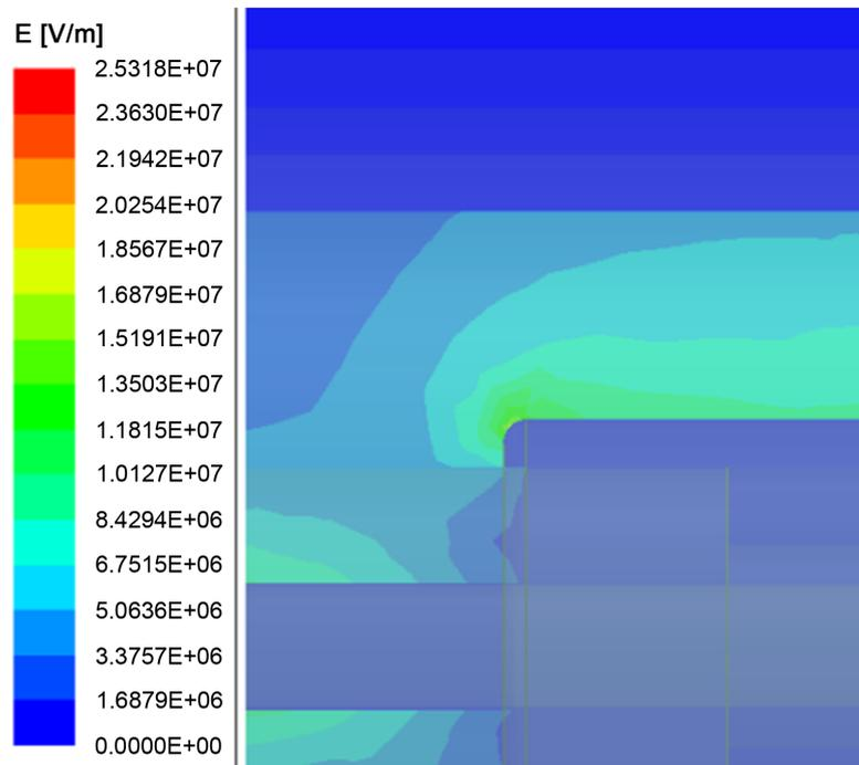
Figure 25. Electric field at the inner shield of 35kV power cable quick-plug connector
