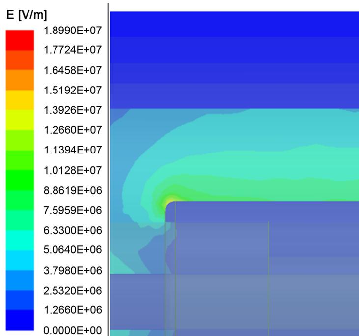
Figure 29. Electric field at the inner shield of 35kV power cable quick-plug connector
