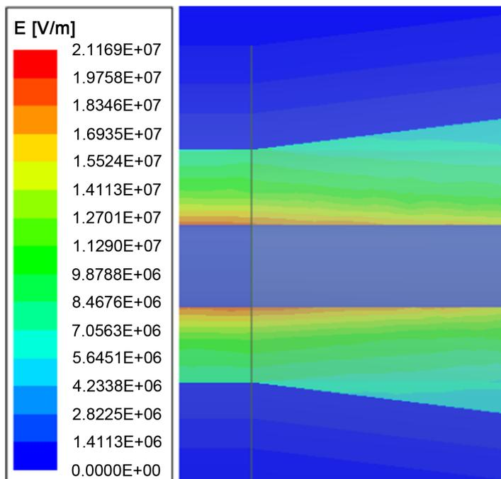
**Figure 10.** Electric field at the stress cone of the 35kV power cable push-in connector
