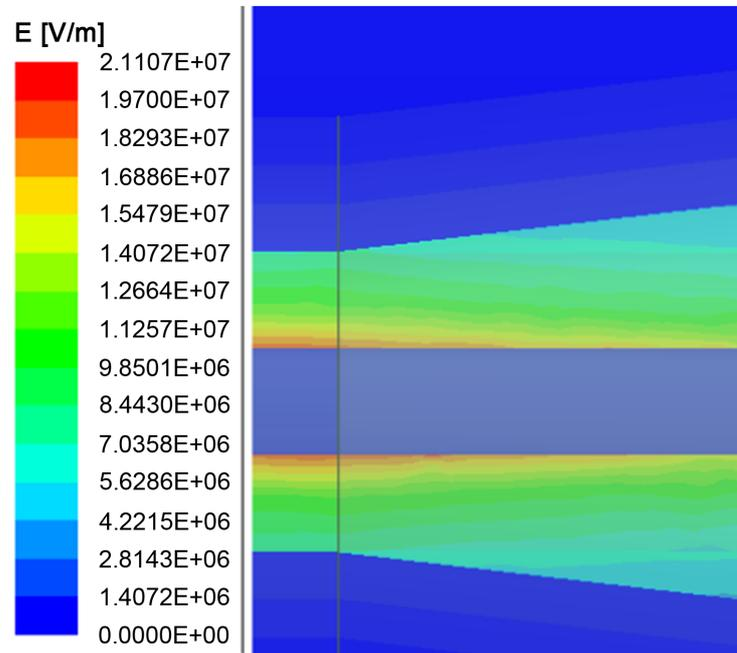
**Figure 12.** Electric field at the stress cone of the 35kV power cable push-in connector
