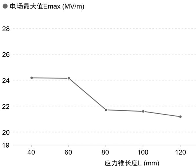
**Figure 11.** Influence of stress cone length on electric field magnitude
