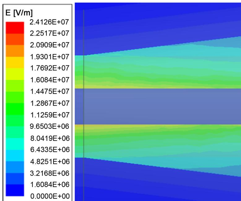
**Figure 7.** Electric field at the stress cone of 35kV power cable push-in connector
