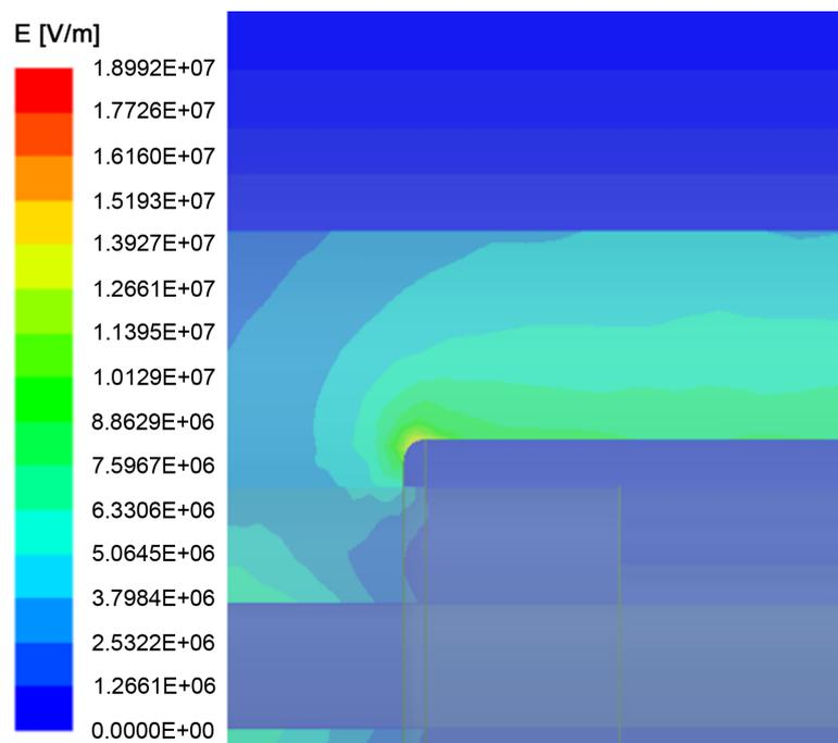
Figure 28. Electric field at the inner shield of 35kV power cable quick-plug connector
