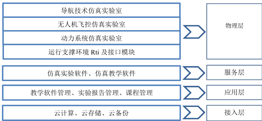
Figure 2. Structure diagram of cloud computer simulation teaching platform 图 2. 云计算仿真教学平台结构图
