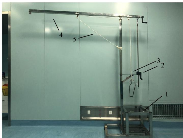
**Figure 1.** (1) Base; (2) Platform; (3) Lifting component; (4) Traction arm; (5) Traction rope
