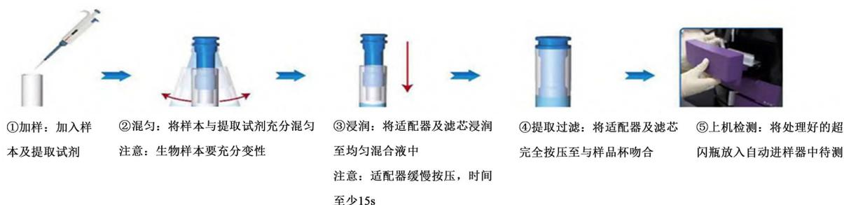
Figure 1. Schematic diagram of in-bottle pre-treatment operation
