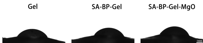
Figure 4. Water contact angle measurements of composite hydrogels. The scale bars: 1 mm
