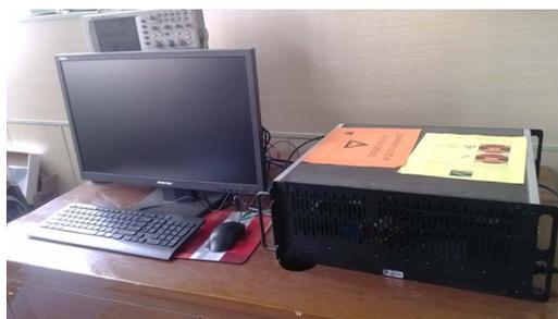
Figure 2. RTLAB hardware in the loop simulation
