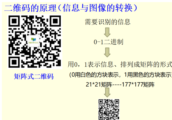
Figure 3. Two-dimensional code generation and recognition principle 图 3. 二维码的生成和识别原理
