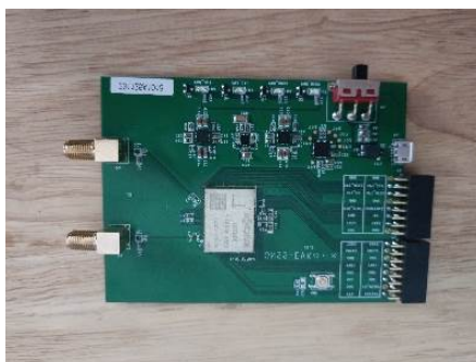
Figure 3. Processed and tested integrated navigation positioning module 图 3. 加工测试好的组合导航定位模组
