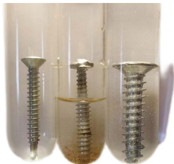
Figure 2. Experimental phenomenon of rust on iron nails 图 2. 铁钉锈蚀的实验现象
