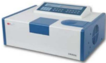
Figure 1. Fluorescence spectrophotometer
