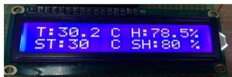
**Figure 15.** Post-PID humidity display
