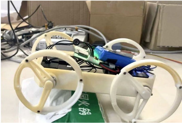
Figure 5. The physical prototype of a wheel-leg deformable robot 图 5. 轮足式变形机器人实体样机
