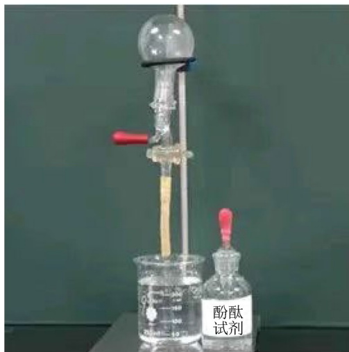
Figure 1. Diagram 1 of the fountain experiment with ammonia gas 图 1. 氨气的喷泉实验装置图 1
