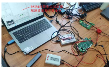
Figure 13. Synchronous Buck built and controlled by students independently 图 13. 学生自主搭建并控制的同步 Buck 图
