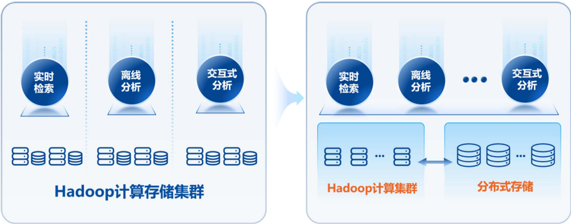
Figure 3. Diagram of the storage and computing separation architecture 图 3. 存算分离架构图
