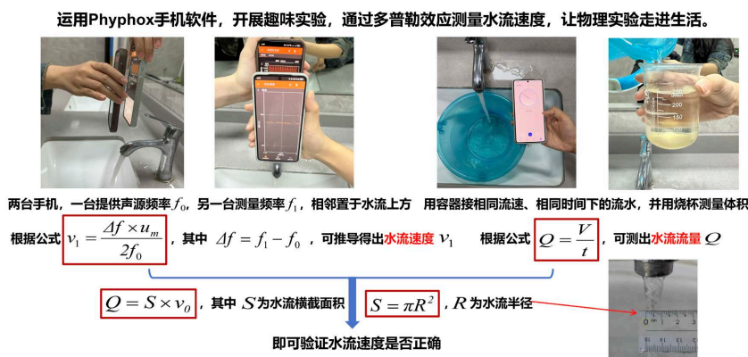
Figure 6. Doppler current measurement principle 图 6. 多普勒水流测速原理
