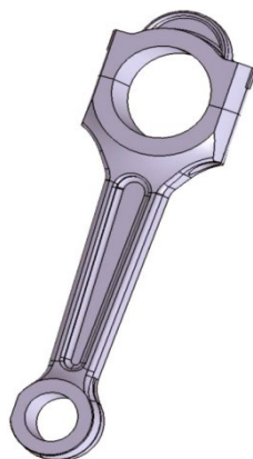
Figure 1. The three-dimensional schematic diagram of an automobile engine connecting rod 图 1. 汽车发动机连杆三维示意图
