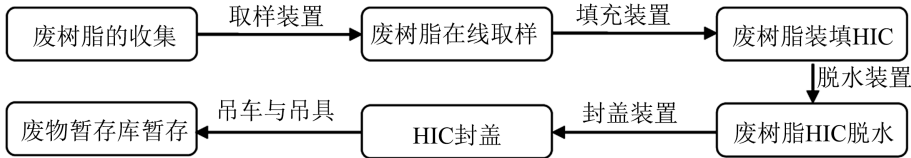
Figure 3. Flow chart of radioactive waste resin treatment [11] 图 3. 放射性废树脂处理流程图[11]
