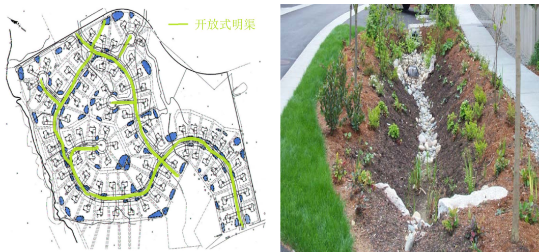
Figure 6. Schematic diagram of village rainwater storage and open channel rainwater collection system 图 6. 村庄雨水蓄滞与开放式明渠雨水收集系统示意图
