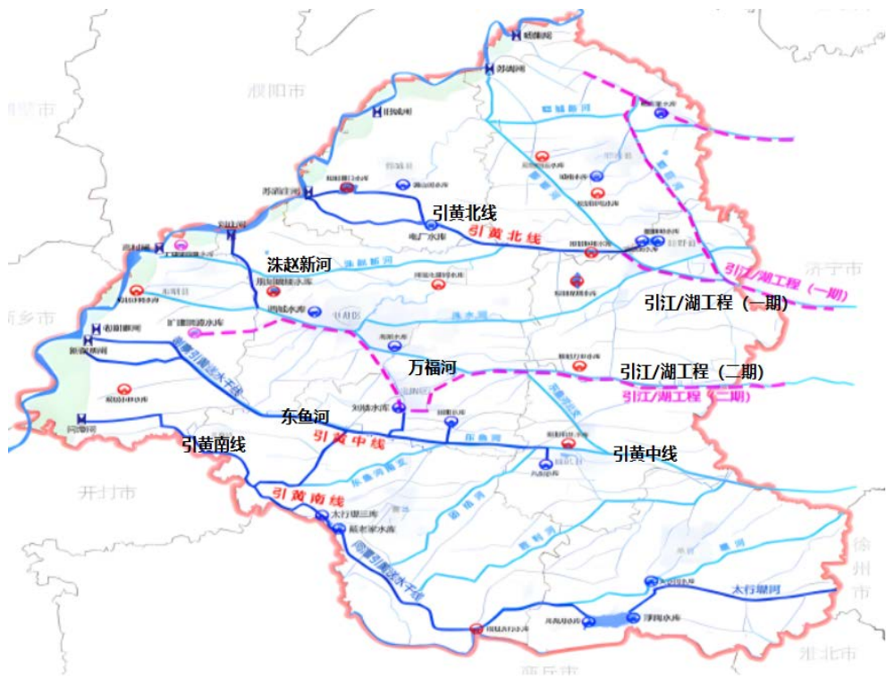
Figure 4. Heze's "Five Horizontal and Six Vertical" main rivers and water diversion projects 图 4. 菏泽“五横六纵”骨干河道和引调水工程
