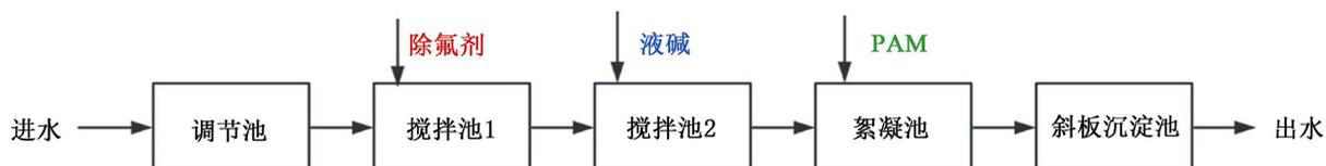
Figure 2. 2# Process flow chart of the fluoride removal system
