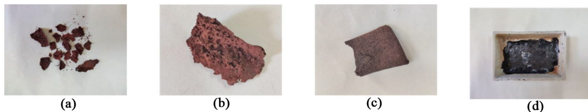
Figure 2. (a) Extremely brittle porous ceramics; (b) Enlarged image of porous ceramics with brittle texture; (c) Samples obtained by sintering at 850°C; (d) Sample obtained by sintering at 1000°C
