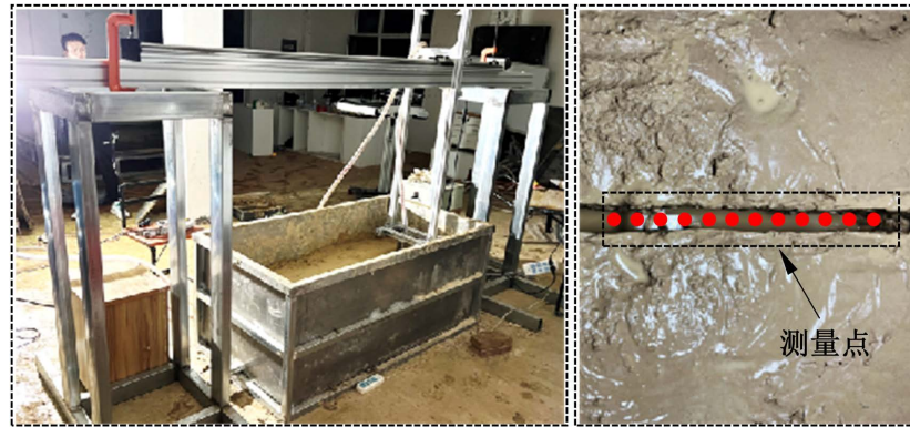
Figure 6. Physical drawing of the device used for the experiment and the grooves made for the experiment. The points where the measurements were taken are labeled in the figure 图 6. 实验所用装置实物图以及实验所开沟槽。图中标注了测量时的点位
