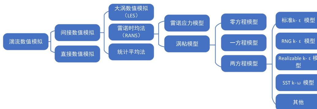
Figure 2. Mainstream turbulence model
