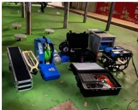
**Figure 2.** Composition of high water level underwater detection equipment for municipal drainage pipelines
