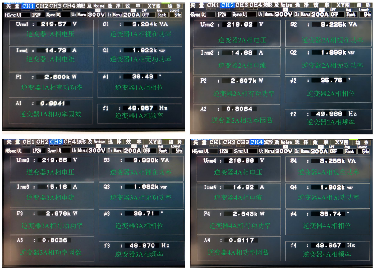
Figure 8. Output data of four inverters under multi-inverter adaptive power decoupling droop control CAN bus
