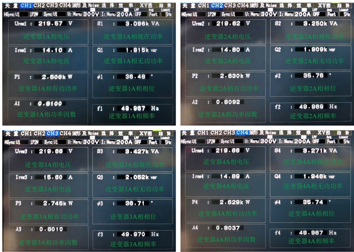
Figure 6. Output data of four inverters under composite control of conventional droop control and virtual impedance 图 6. 传统下垂控制和虚拟阻抗复合控制下的四台逆变器输出数据
