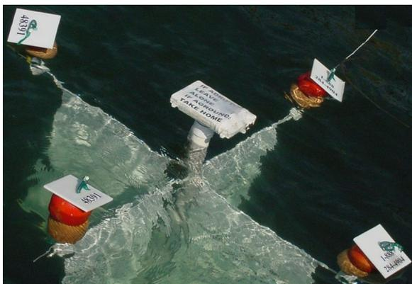
Figure 1. GPS-based ocean drifter
