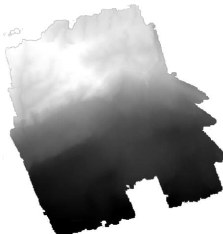
**Figure 5.** Ground points generate DEM
