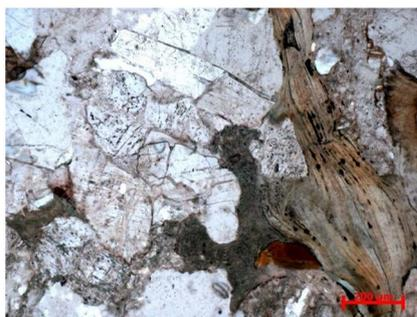
**Figure 7.** The biotite's phenomenon of compression bending and iron removal
