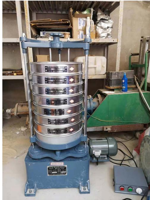
**Figure 2.** Top strike type standard vibrating sieving machine and new standard square hole test sieves
