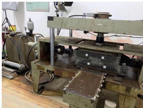
Figure 1. Large-scale interface shearing apparatus
