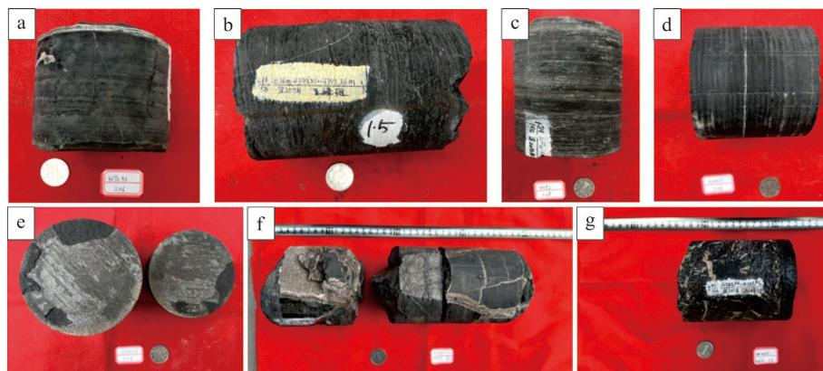
**Figure 2.** Types of natural fractures at core scale. (a) High-angle seam (b) High-angle joints, filled with calcite; (c) High-angle joint, filled with calcite; (d) Bedding joint, filled with calcite; (e) Bedding joints, filled with pyrite and calcite; (f) Develop multi-stage fractures, filled with calcite; (g) Develop multi-stage fractures, filled with calcite
